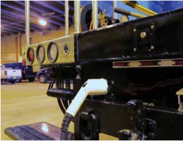
This photo shows a close up of the plug-in power unit.
