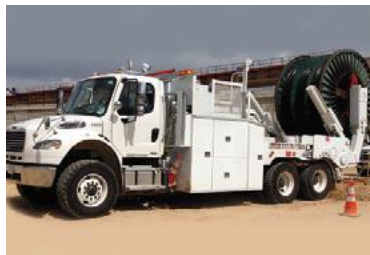
Cable Handling/Pulling Trucks
