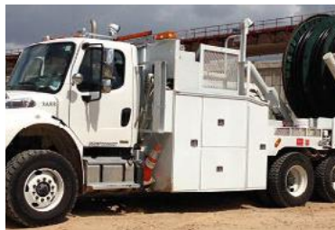
Cable Handling/Pulling Trucks
